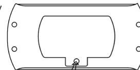
open the battery compartment cover by unscrewing the screw, then push the clip in the direction indicated by arrow.
