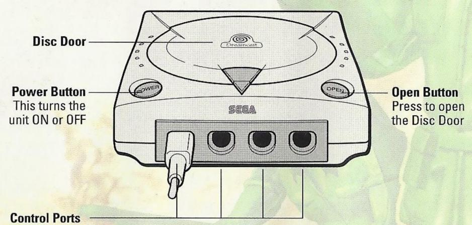
Use these ports to connect the Sega Dreamcast Controller or other peripheral equipment. From left to right are Control Port A, Control Port B, Control Port C, and Control Port D. Use each port to connect controllers for players 1 to 4 respectively.
