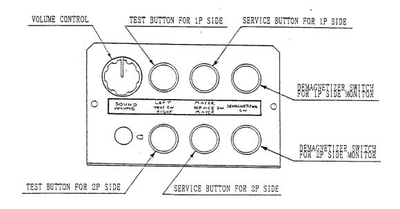
Open the Coin Chute Door, and the SW unit shown will appear. The functioning of each SW is as follows:
