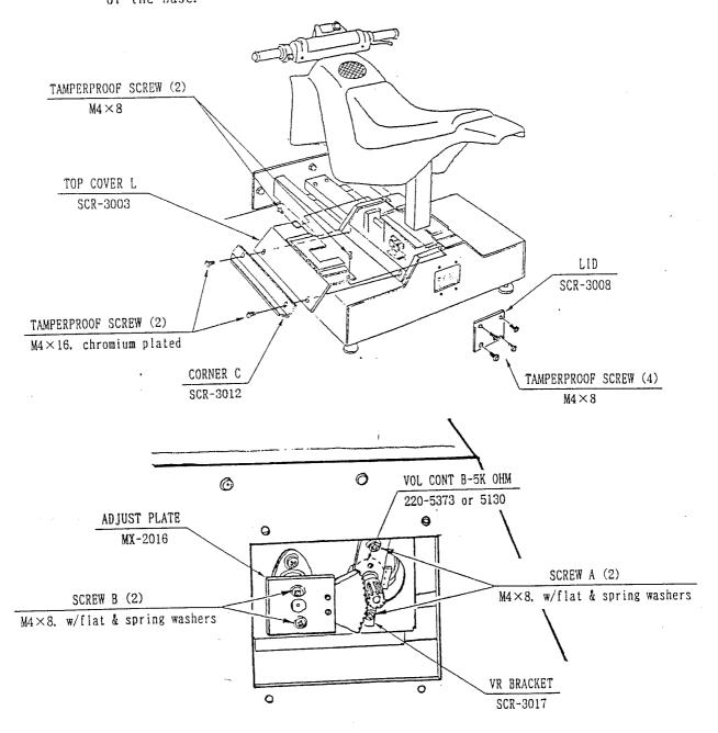
\* When the Bike is inclined to the right and left, if the VR is not turned in excess of the MAX. turning limit or the gears are not disengaged, then no adjustments are required.
