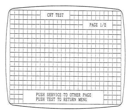
When adjusting the monitor size, be careful that grids do not go off of the screen.
