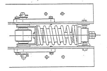
Take off the COVER, check the SPRING UNIT and thoroughly apply grease to the inside of the GUIDE PLATE (plastic).
