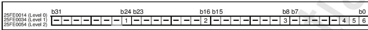
Figure 3.10 Level 2-0 DMA Mode, Address Update, Start Factor Select Register (Register : D0MD, D1MD, D2MD) Initial Value 00000007H
