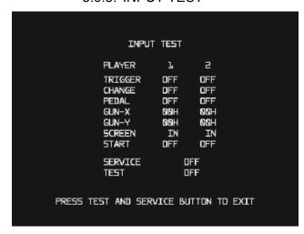
Selecting the INPUT TEST on the game test mode menu screen causes the screen (on which each switch is tested) to be displayed. Press each switch. If the display beside each switch indicates "ON," the switch and wiring connections are satisfactory.
