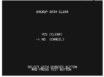
To clear data, use the SERVICE Button to move the cursor to YES (CLEAR) and then press the TEST Button. When the data has been cleared, the message "COMPLETED" will be displayed.
