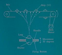
The torpedo track as it nears the ship aimed at has the possibility of changing course in one of two directions due to the action of the mixer unit, there is a position however that as the player picks-up skill he can manage a hit more often by taking into consideration the speed of the moving target and adjusting his aim accordingly.
