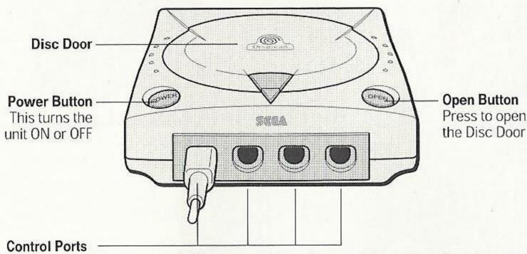
Use these ports to connect the Dreamcast Controller or other peripheral equipment. From left to right are Control Port A, Control Port B, Control Port C, and Control Port D. Use each port to connect controllers for players 1 to 4 respectively.
