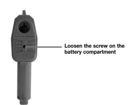
On the front of the Menacer loosen the screw on the battery compartment and insert four (4) "AA" batteries as indicated inside the compartment (alkaline batteries recommended). Replace the battery compartment door.
