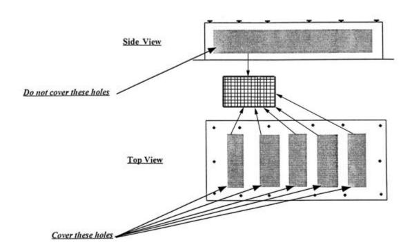
TO AVOID POSSIBLE DAMAGE DUE TO LIQUID SPILLAGE, COVER HOLES ON THE TOP COVER OF THE PCB CAGE ASSEMBLY WITH VINYL PACKING TAPE. BE SURE TO COMPLETELY COVER ALL OF THE SMALL HOLES ON THE TOP OF THE CAGE. PLACE TAPE BOTH INSIDE AND OUTSIDE OF THE LID. DO NOT COVER ANY OF THE SIDE HOLES ON THE CAGE!!!!!! THESE ARE NEEDED TO ASSURE THE PCB IS PROPERLY VENTILATED.
