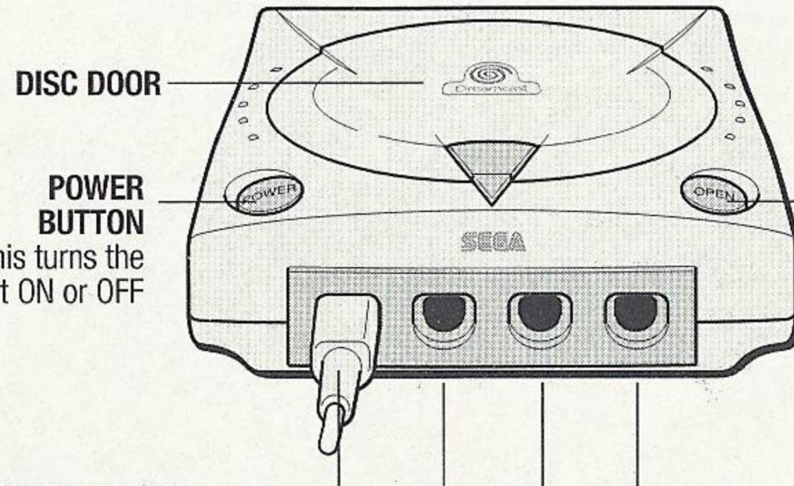
**CONTROL PORT A, CONTROL PORT B, CONTROL PORT C, AND CONTROL PORT D.** Use each port to connect controllers for players 1 to 4 respectively.
