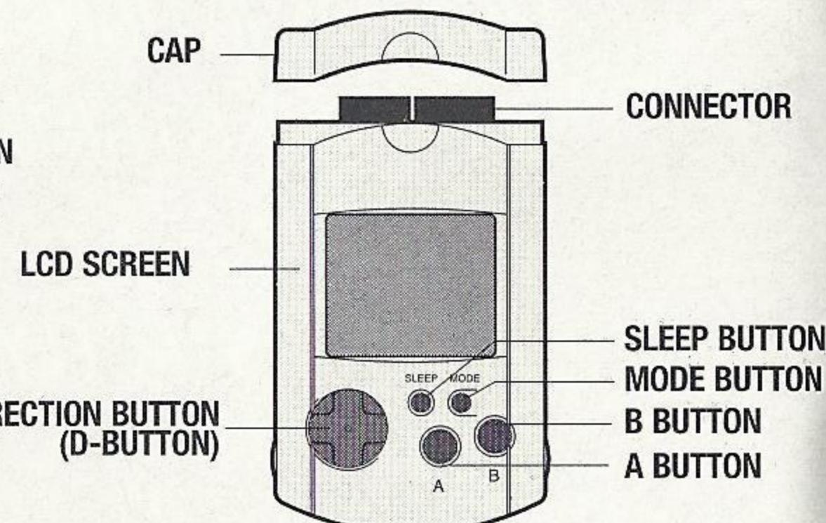
Never disconnect the VMU / VMs while performing a battle or exchanging data when connected to another VMU/VM. Also note that leaving two VMU / VMs connected for a long period of time will considerably shorten the life of the batteries.
